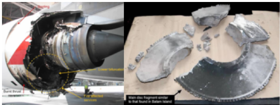
图 3 Trent 900 中压涡轮超转非包容失效 Fig. 3 Uncontained failure of Trent 900 intermediate pressure turbine overspeed
